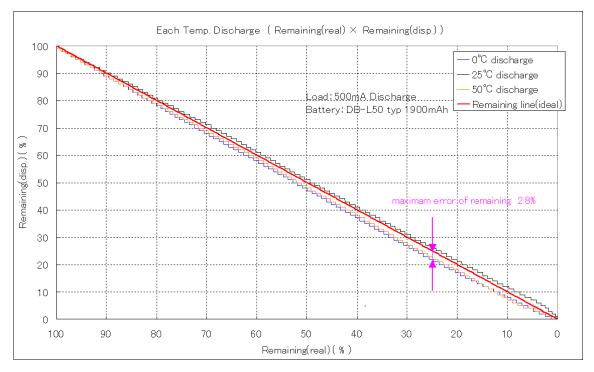
Figure 2 Discharge Characteristics by Temperature Change
