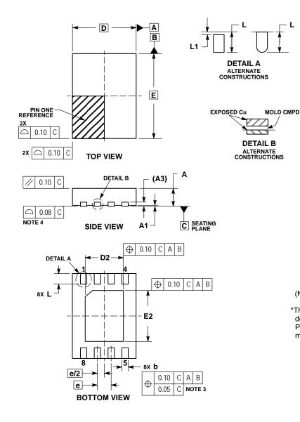
NOTES: 1. DIMENSIONING AND TOLERANCING PER ASME Y14.5M, 1994. 2. CONTROLLING DIMENSION: MILLIMETERS. 3. DIMENSION & APPLIES TO PLATED TERMINAL AND IS MEASURED BETWEEN 0.15 AND 0.30mm FROM THE TERMINAL TIP. 4. PROFILE TOLERANCE APPLIES TO THE EXPOSED PAD AS WELL AS THE LEADS.
