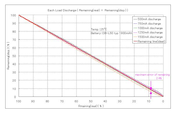
Figure 3 Discharge Characteristics by Load Change
