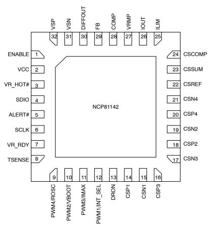
Figure 2. NCP81142 Pin Configurations
