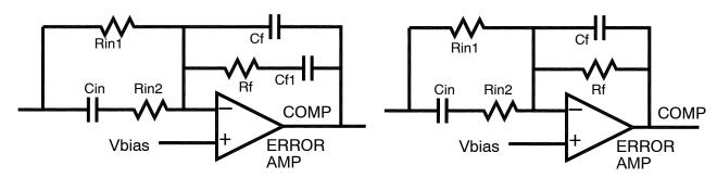
Figure 4. Traditional Type 3 External Compensation
