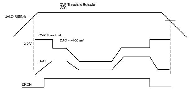
Figure 13. OVP Threshold Behavior
