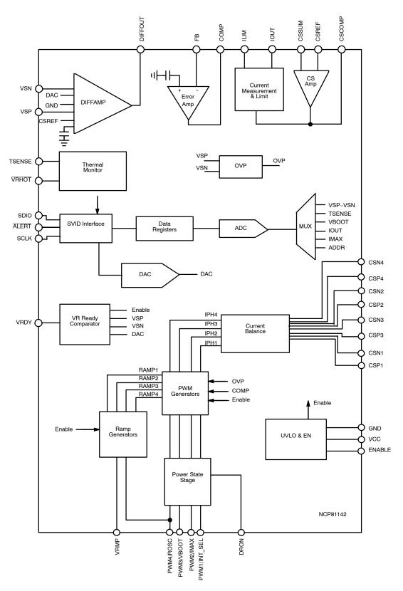
Figure 1. Block Diagram for NCP81142
