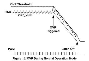
During start up, the OVP threshold is set to 2.9 V. This allows the controller to start up without false triggering the OVP.
