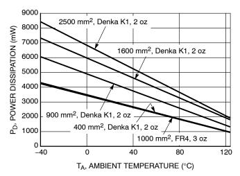
Figure 6. Power Dissipation vs. Ambient Temperature @  $T_J = 175$ °C
