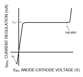
Figure 1. CCR Voltage-Current Characteristic
