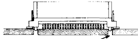
Tab for positioning on the PC board. Suitable for both manual and automatic insertion.
