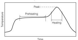
For soldering (Example: Sn/Pb)
