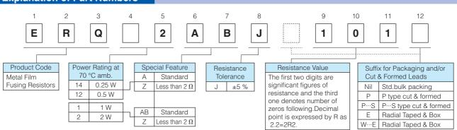
The above example shows a standard Metal Film Fusing Resistors, 2 W power rating, resistance value of 100  $\Omega$ , tolerance of ±5 %, and package of standard bulk packing.
