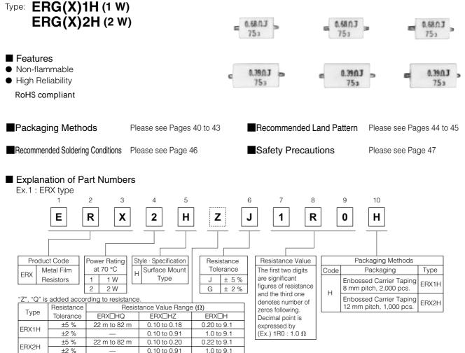
The above example 1 shows a metal film resistor SMD type, 2 W power rating, resistance value of 1.0 Ω, tolerance ±5 %, and embossed taping.
