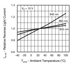
Fig. 2 - Relative Reverse Light Current vs. Ambient Temperature
