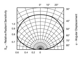
Fig. 7 - Relative Radiant Sensitivity vs. Angular Displacement
