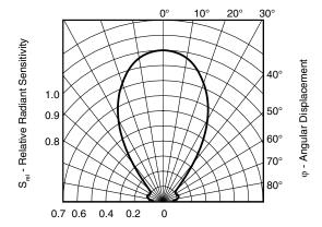
Fig. 6 - Relative Radiant Sensitivity vs. Angular Displacement
