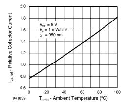
Fig. 7 - Relative Collector Current vs. Ambient Temperature
