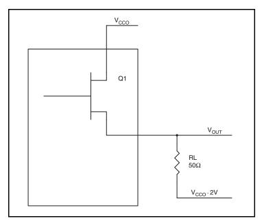
Figure 7. LVPECL Driver Circuit and Termination
