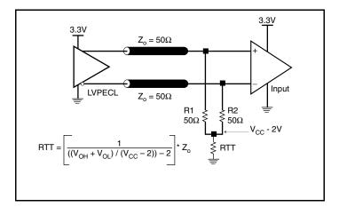
Figure 4A. 3.3V LVPECL Output Termination
