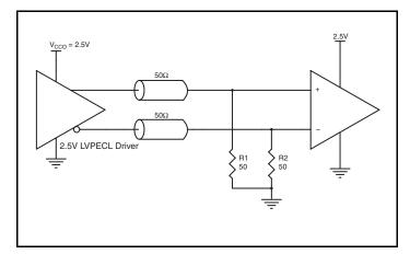
Figure 5C. 2.5V LVPECL Driver Termination Example
