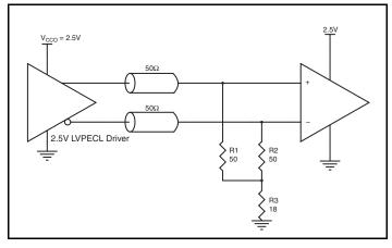
Figure 5B. 2.5V LVPECL Driver Termination Example
