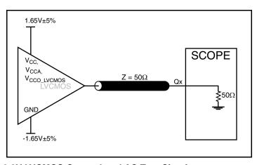
3.3V LVCMOS Output Load AC Test Circuit
