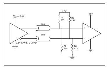
Figure 5A. 2.5V LVPECL Driver Termination Example
