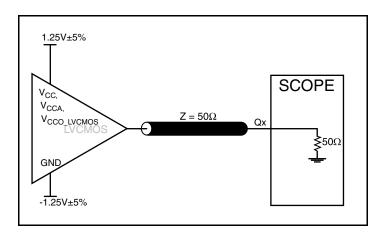
2.5V LVCMOS Output Load AC Test Circuit
