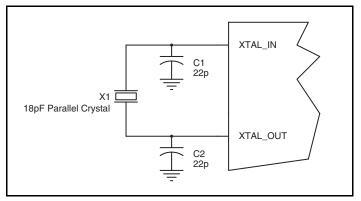
Figure 2. Crystal Input Interface
