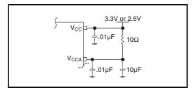
Figure 1. Power Supply Filtering
