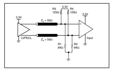
Figure 4B. 3.3V LVPECL Output Termination
