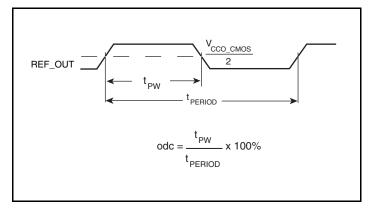
LVCMOS Output Duty Cycle/Pulse Width/Period
