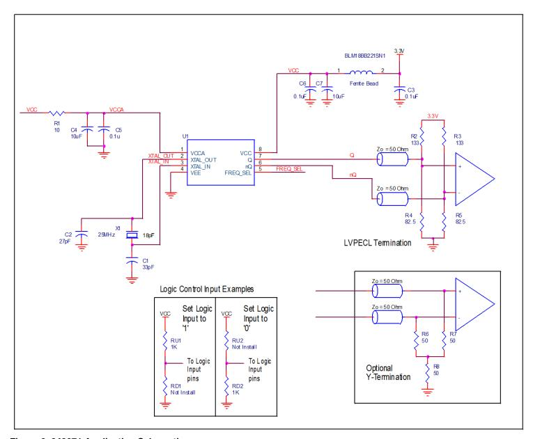
Figure 6. 843071 Application Schematic
