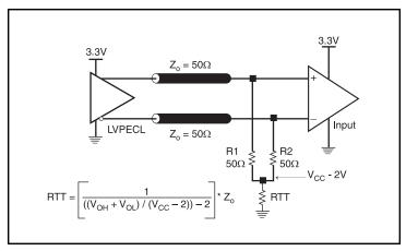
Figure 4A. 3.3V LVPECL Output Termination
