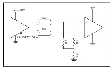
Figure 5B. 2.5V LVPECL Driver Termination Example
