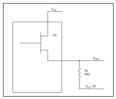
Figure 6. LVPECL Driver Circuit and Termination
