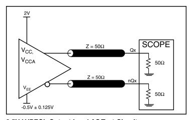
2.5V LVPECL Output Load AC Test Circuit
