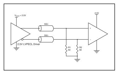
Figure 5C. 2.5V LVPECL Driver Termination Example
