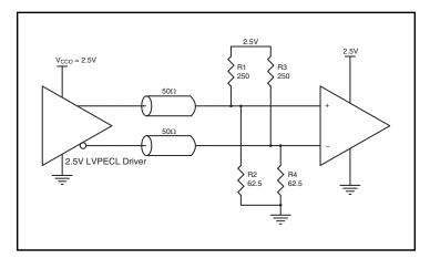
Figure 5A. 2.5V LVPECL Driver Termination Example
