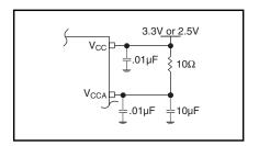
Figure 1. Power Supply Filtering
