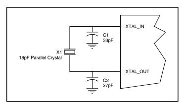
Figure 2. Crystal Input Interface
