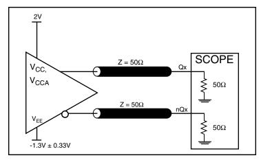
3.3V LVPECL Output Load AC Test Circuit
