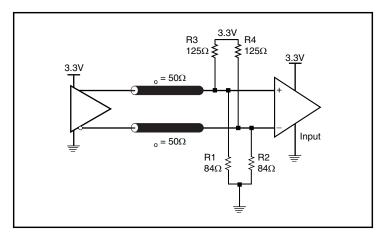
Figure 4B. 3.3V LVPECL Output Termination
