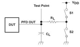
Figure 3. PFD Output Test Condition
