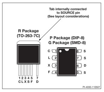
Figure 2. Pin Configuration (Top View).
