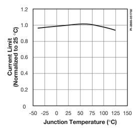
Figure 37. Internal Current Limit vs. Temperature.
