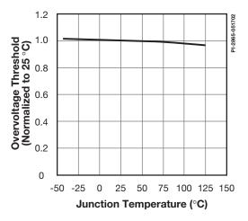
Figure 39. Overvoltage Threshold vs. Temperature.
