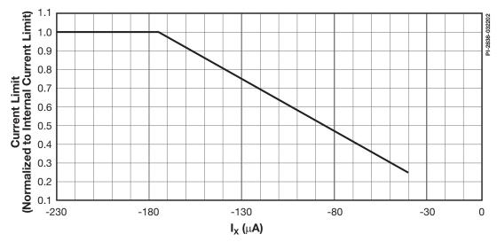
Figure 34. Current Limit vs. EXTERNAL CURRENT LIMIT Pin Current.
