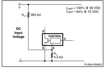
Figure 16. Current Limit Reduction with Line Voltage.
