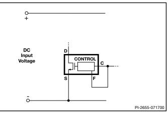
Figure 9. 400 kHz Frequency Operation.
