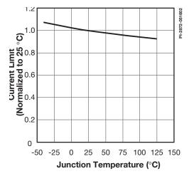
Figure 38. External Current Limit vs. Temperature with  $R_{\parallel} = 12 \text{ k}\Omega$ .
