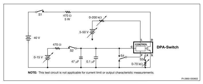
Figure 33. DPA-Switch General Test Circuit.
