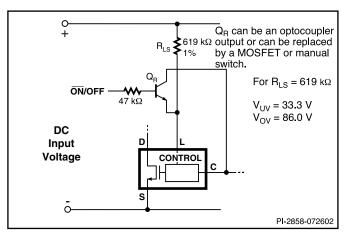
Figure 22. Active-off Remote ON/OFF with LINE-SENSE.
