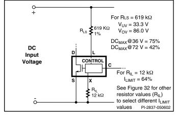
Figure 23. Line-Sensing and Externally Set Current Limit.
