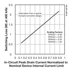
Figure 51. Typical Switching Loss.
