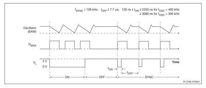
Figure 6. Synchronization Timing Diagram.
