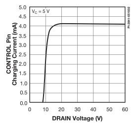
Figure 45. I<sub>c</sub> vs. DRAIN Voltage.
