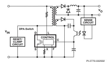
Figure 1. Typical Forward Converter Application.
