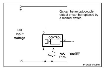
Figure 17. Active-on (Fail Safe) Remote ON/OFF.
