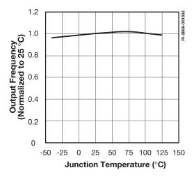
Figure 36. Frequency vs. Temperature.
