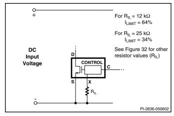
Figure 15. Externally Set Current Limit.
