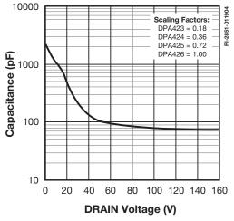
Figure 50. C<sub>oss</sub> vs. DRAIN Voltage.
