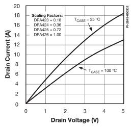
Figure 48. Output Characteristics.
