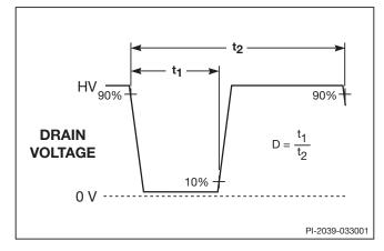
Figure 30. Duty Cycle Measurement.
