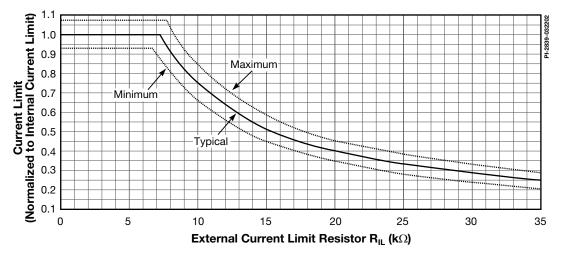
Figure 35. Current Limit vs. External Current Limit Resistance.
