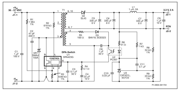
Figure 26. A Cost Effective 6.6 W, 3.3 V Flyback DC-DC Converter.
