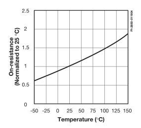
Figure 49. On-Resistance vs. Temperature.
