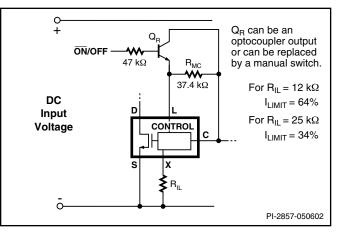
Figure 20. Active-off Remote ON/OFF with Externally Set Current Limit.
