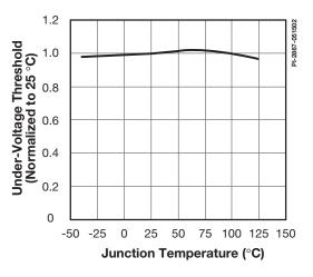
Figure 40. Undervoltage Threshold vs. Temperature.
