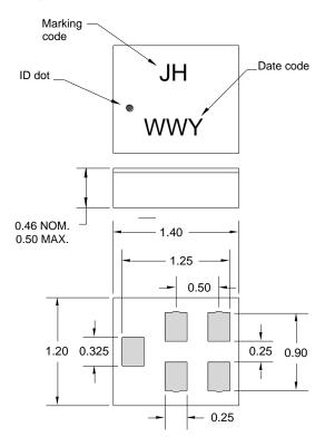
Package Style: CSP-5BT Dimensions: 1.40 x 1.20 x 0.46 mm
