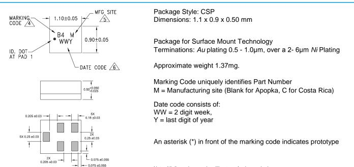
Note: All dimensions are in millimeters. Angles are in degrees
