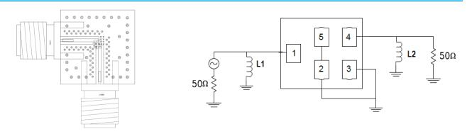
Notes: Matching component values shown are for the specified TriQuint evaluation board. Value adjustment may be required in end user product circuits depending on component manufacturer and PCB material.
