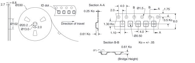
Standard T/R size=15,000 units/reel. All dimensions are in millimeters.
