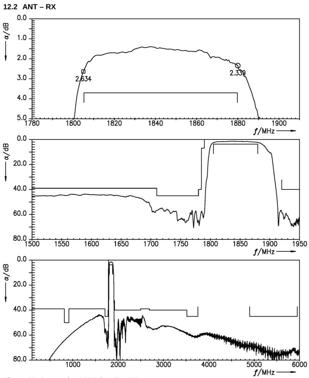
**Figure 11:** Attenuation LTE B3 ANT – RX.
