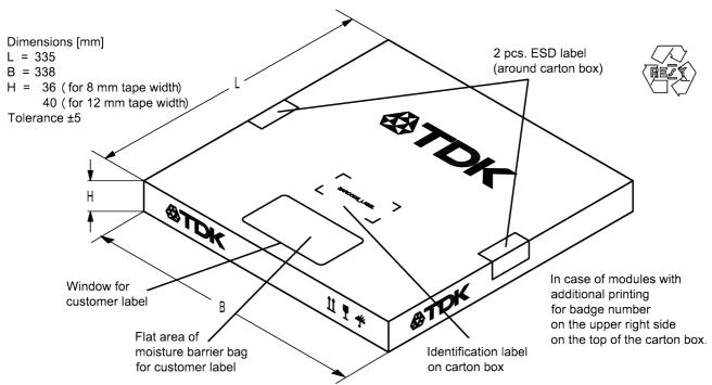
Figure 24: Drawing of folding box for reel with diameter of 330 mm.
