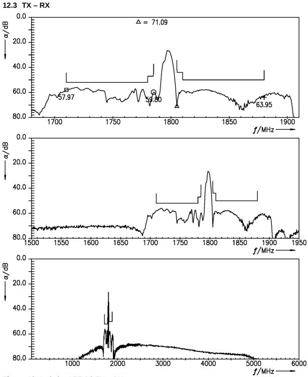
Figure 12: Isolation LTE B3 TX – RX.
