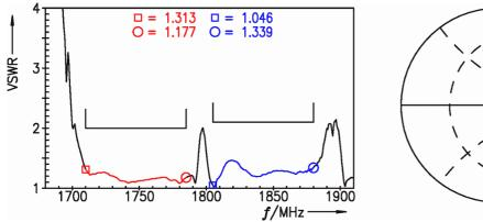
Figure 14: Reflection coefficient LTE B3 at ANT port (TX and RX frequencies).
