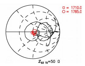
Figure 13: Reflection coefficient LTE B3 at TX port.
