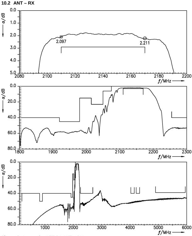
**Figure 5:** Attenuation LTE B1 ANT – RX.
