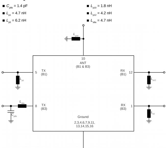
Figure 3: Schematic of matching circuit.
