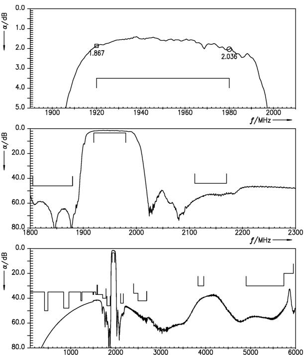
Figure 4: Attenuation LTE B1 TX – ANT.
