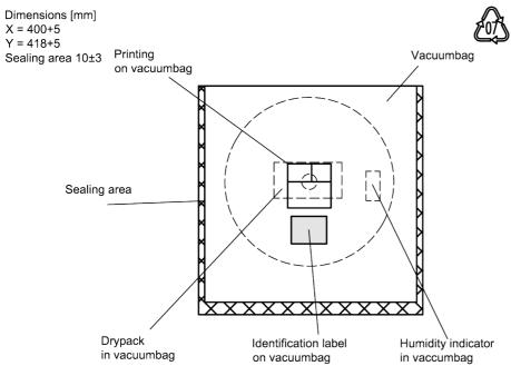
Figure 23: Drawing of moisture barrier bag (MBB) for reel with diameter of 330 mm.
