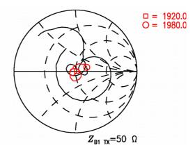
Figure 7: Reflection coefficient LTE B1 at TX port.
