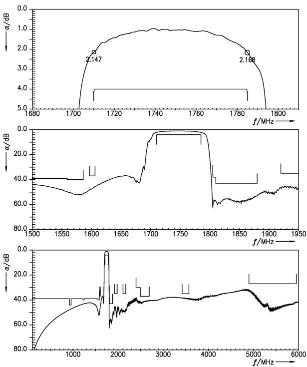
Figure 10: Attenuation LTE B3 TX – ANT.
