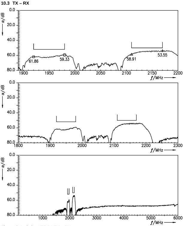
**Figure 6:** Isolation LTE B1 TX – RX.
