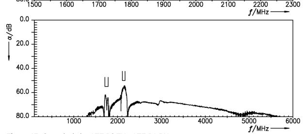
Figure 17: Cross-isolation LTE B3 TX - LTE B1 RX.
