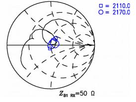
Figure 9: Reflection coefficient LTE B1 at RX port.
