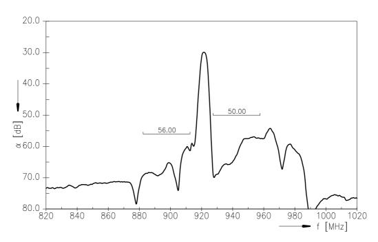
Frequency Response TX - RX (Power transfer function, common mode)
