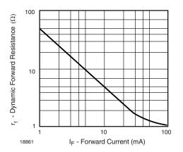
Fig. 4 - Dynamic Forward Resistance vs. Forward Current
