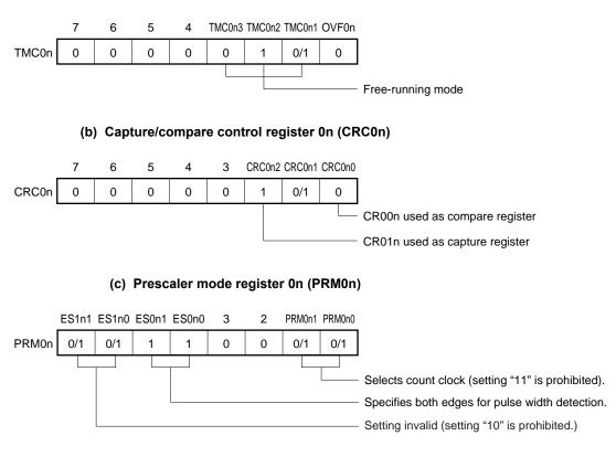
Cautions 1. Only 16-bit timer/event counter 00 can use the pulse width measurement of 78K0/FC2.
