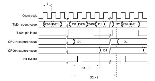
Figure 7-45. Timing of Pulse Width Measurement Operation by Means of Restart (with Rising Edge Specified)
