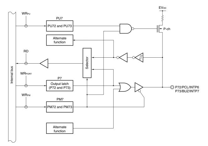
Figure 5-17. Block Diagram of P72 and P73
