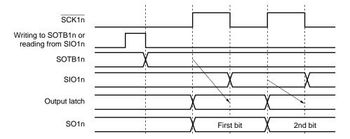
The first bit is directly latched by the SOTB1n register to the output latch at the falling (or rising) edge of  $\overline{SCK1n}$ , and output from the SO1n pin via an output selector. Then, the value of the SOTB1n register is transferred to the SIO1n register at the next rising (or falling) edge of  $\overline{SCK1n}$ , and shifted one bit. At the same time, the first bit of the receive data is stored in the SIO1n register via the SI1n pin.
