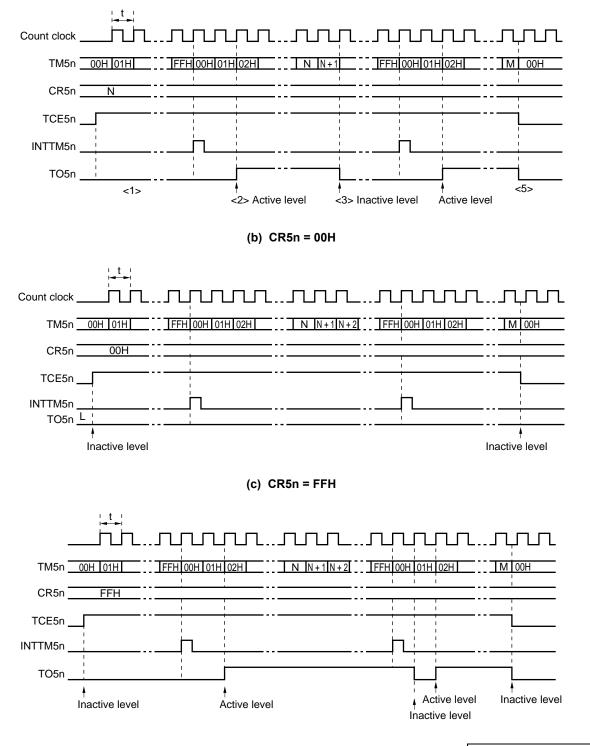
Remarks 1. <1> to <3> and <5> in Figure 8-14 (a) correspond to <1> to <3> and <5> in PWM output operation in 8. 4. 4 (1) PWM output basic operation.
