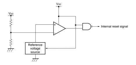
Figure 21-1. Block Diagram of Power-on-Clear Circuit
