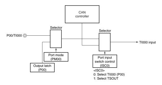
Figure 16-36. Port Input Switch Control
