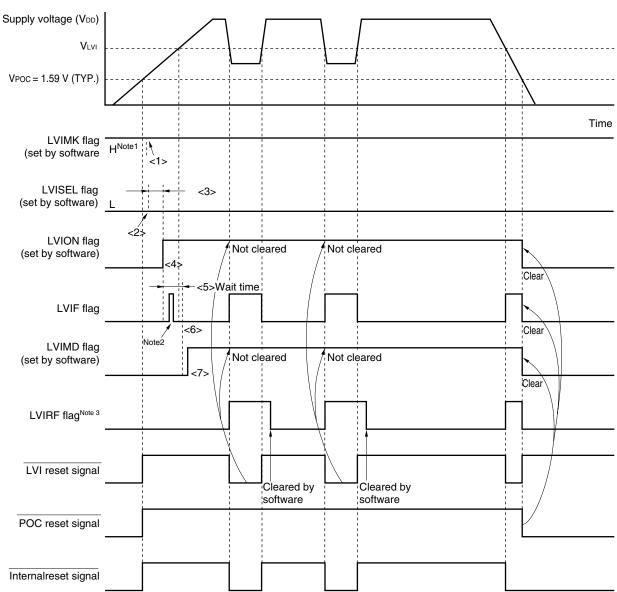
(Detects Level of Supply Voltage (VDD)) (1/2)
