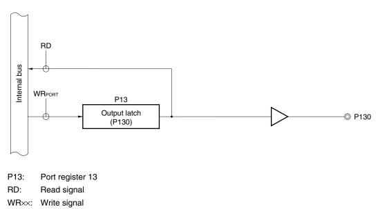
**Remark** When reset is effected, P130 outputs a low level. If P130 is set to output a high level before reset is effected, the output signal of P130 can be dummy-output as the CPU reset signal.
