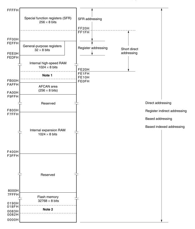
Figure 3-7. Correspondence Between Data Memory and Addressing (µPD78F0881A, 78F0884A)
