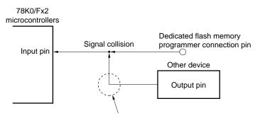
In the flash memory programming mode, the signal output by the device collides with the signal sent from the dedicated flash memory programmer. Therefore, isolate the signal of the other device.
