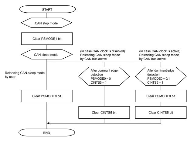
**Remark** "In case CAN clock is disabled": By means of the CPU standby mode, the CAN module clock has been switched off, and the CAN module is in sleep mode.
