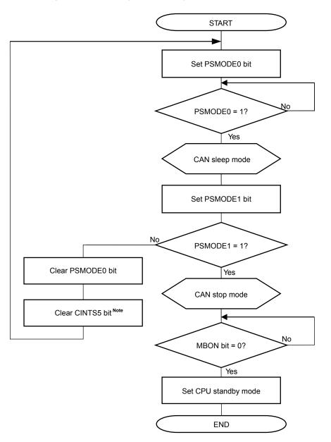
Figure 16-62. Setting CPU Standby (from CAN Stop Mode)
