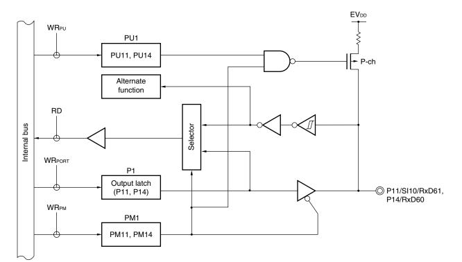
Figure 5-4. Block Diagram of P11 and P14
