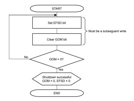
Figure 16-59. Forced Shutdown Process
