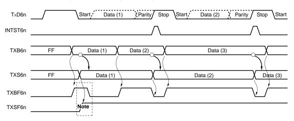
Figure 14-26. Timing of Starting Continuous Transmission
