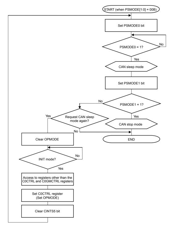
Figure 16-54. Setting CAN Sleep Mode/Stop Mode
