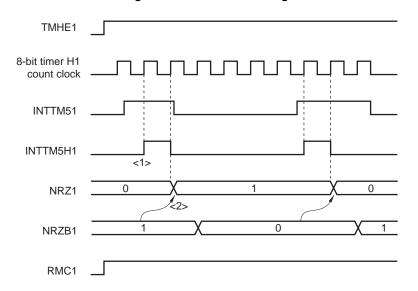
Figure 9-13. Transfer Timing
