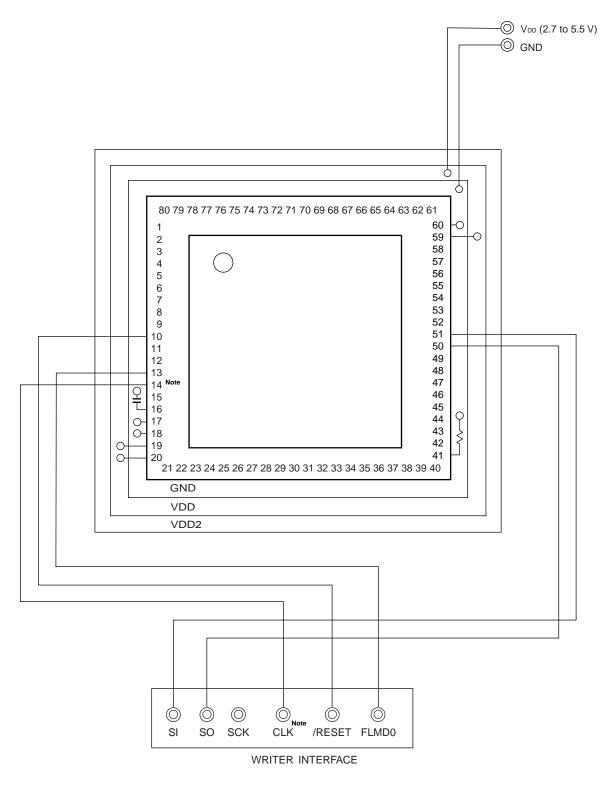
**Note** The above figure illustrates an example of wiring when using the clock output from the PG-FP5, FL-PR5, PG-FP4 or FL-PR4.
