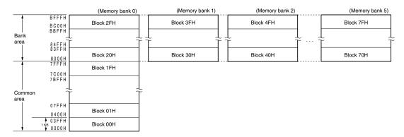
Correspondence between the address values and block numbers in the flash memory are shown below.
