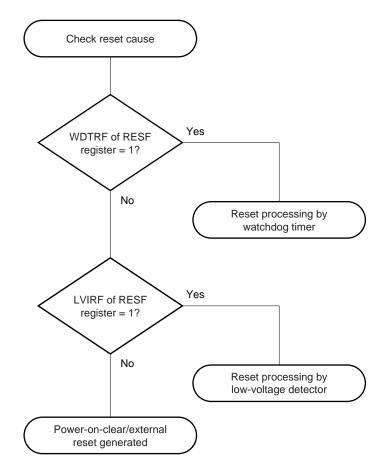
Figure 21-3. Example of Software Processing After Release of Reset (2/2)
