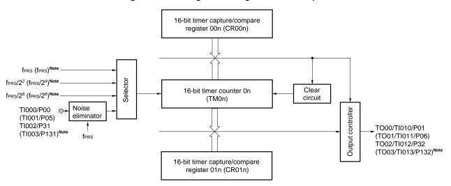
Figure 7-34. Configuration Diagram of PPG Output
