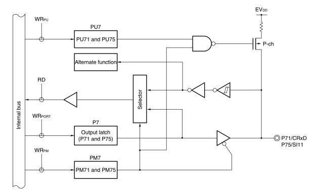
Figure 5-16. Block Diagram of P71 and P75
