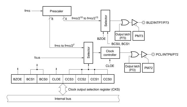
Figure 12-1. Block Diagram of Clock Output/Buzzer Output Controller
