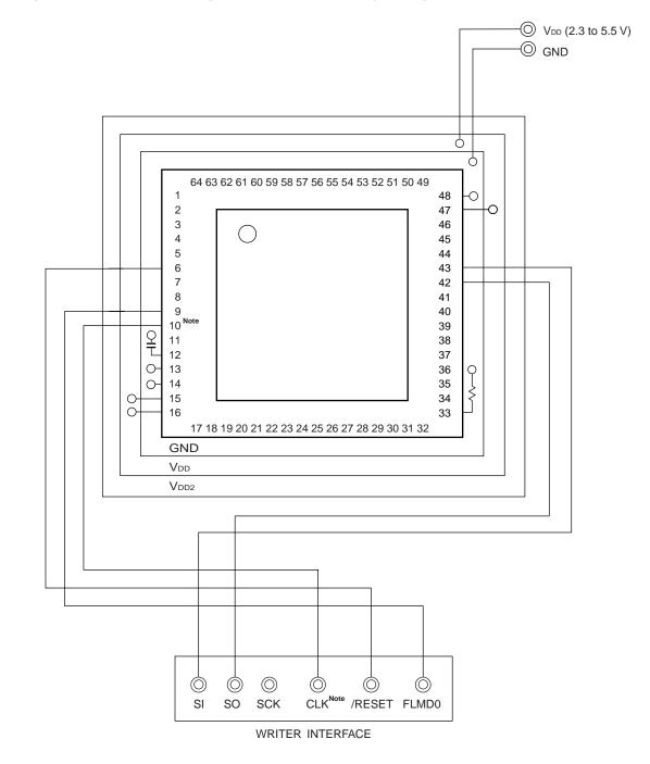
Figure 24-8. Example of Wiring Adapter for Flash Memory Writing in UART (UART60) Mode (78K0/FE2)
