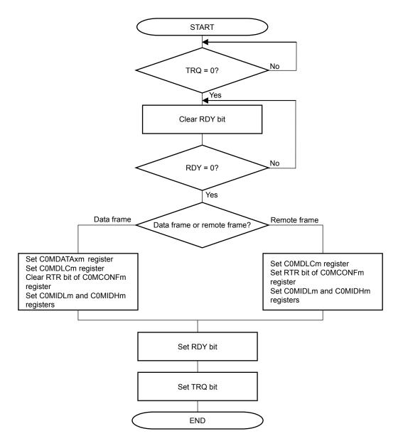
Figure 16-42. Message Transmit Processing
