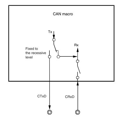
Figure 16-34. CAN Module Terminal Connection in Self-test Mode
