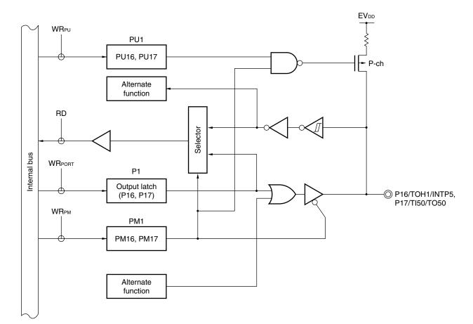
Figure 5-7. Block Diagram of P16 and P17
