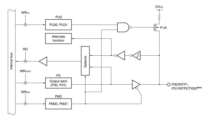
Figure 5-8. Block Diagram of P30 and P31
