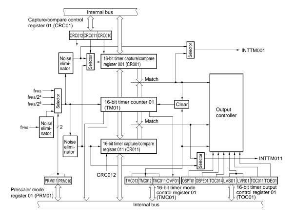
Figure 7-2. Block Diagram of 16-Bit Timer/Event Counter 01 (µPD78F0881A, 78F0882A, 78F0883A of 78K0/FC2)
