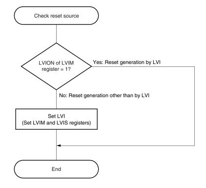
Figure 22-9. Example of Software Processing After Reset Release (2/2)
