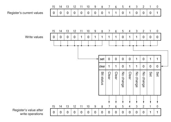
Figure 16-24. 16-Bit Data during Write Operation
