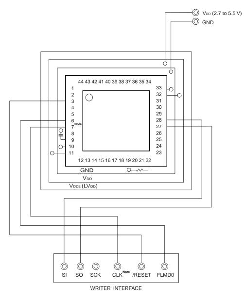
Figure 23-4. Example of Wiring Adapter for Flash Memory Writing in UART (UART60) Mode (µPD78F0881A, 78F0882A, 78F0883A of 78K0/FC2)
