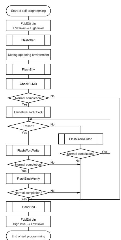
Figure 24-22. Flow of Self-Programming (Rewriting Flash Memory)
