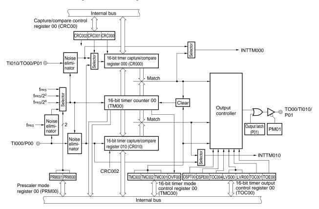
Figure 7-1. Block Diagram of 16-Bit Timer/Event Counter 00
