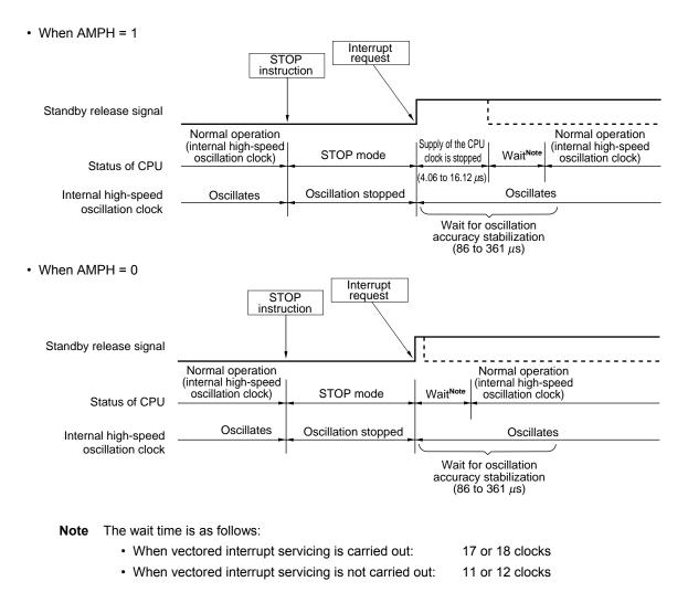
**Remark** The broken lines indicate the case when the interrupt request that has released the standby mode is acknowledged.
