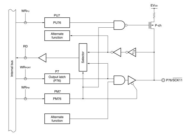
Figure 5-18. Block Diagram of P76
