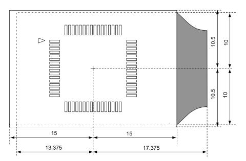
Figure B-4. The Restriction Domain on a Target System (Case of 64-pin GK Package)
