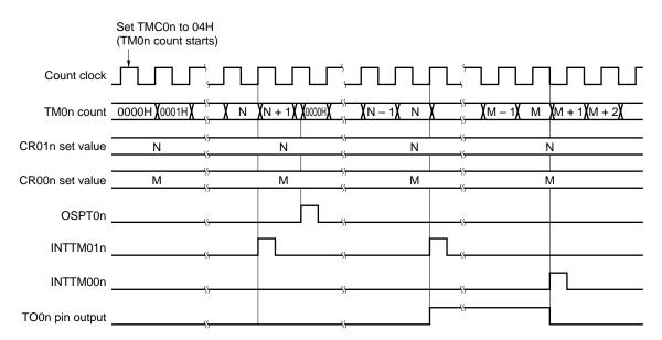
Figure 7-52. Timing of One-Shot Pulse Output Operation with Software Trigger
