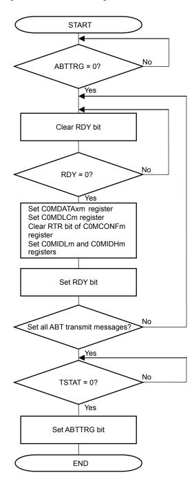
Figure 16-43. ABT Message Transmit Processing
