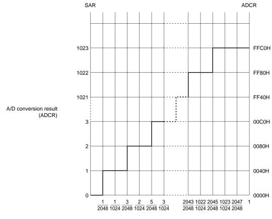
Figure 13-13 shows the relationship between the analog input voltage and the A/D conversion result.
