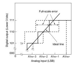
Figure 13-20. Differential Linearity Error
