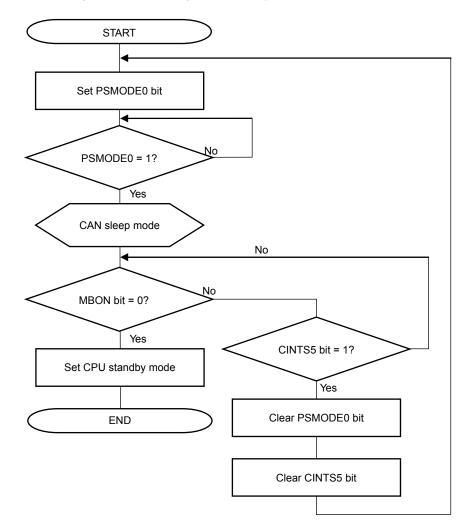
Figure 16-61. Setting CPU Standby (from CAN Sleep Mode)
