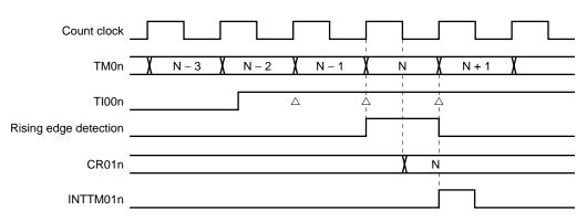
Figure 7-36. CR01n Capture Operation with Rising Edge Specified
