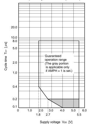
TCY vs. VDD (Main System Clock Operation)
