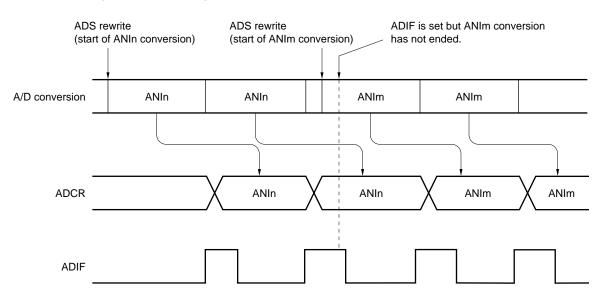
Figure 13-22. Timing of A/D Conversion End Interrupt Request Generation
