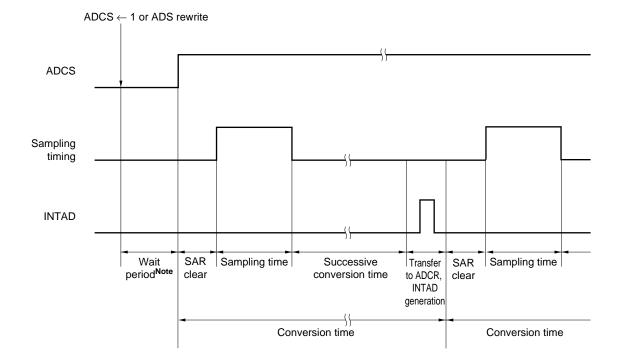
Figure 13-5. A/D Converter Sampling and A/D Conversion Timing
