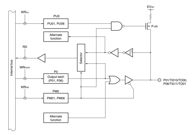
Figure 5-2. Block Diagram of P01 and P06
