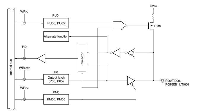
Figure 5-1. Block Diagram of P00 and P05
