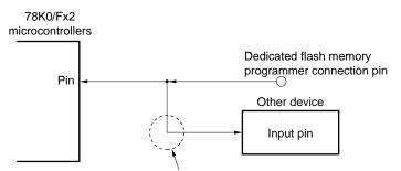
If the signal output by the dedicated flash memory programmer in the flash memory programming mode affects the other device, isolate the signal of the other device.
