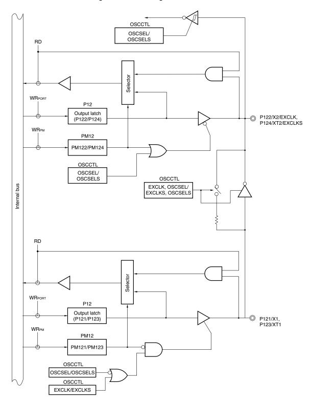
Figure 5-22. Block Diagram of P121 to P124
