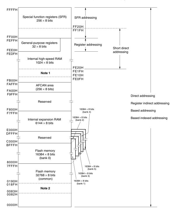
Figure 3-11. Correspondence Between Data Memory and Addressing (µPD78F0890A, 78F0893A, 78F0895A)
