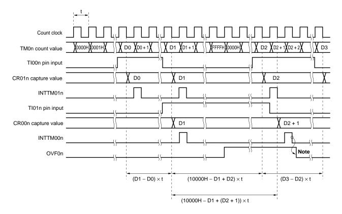
Figure 7-41. Timing of Pulse Width Measurement Operation with Free-Running Counter (with Both Edges Specified)
