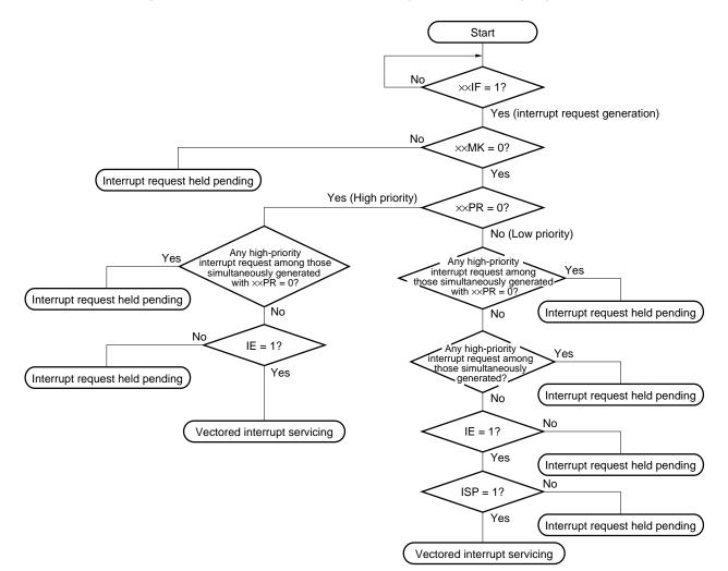
Figure 17-10. Interrupt Request Acknowledgement Processing Algorithm
