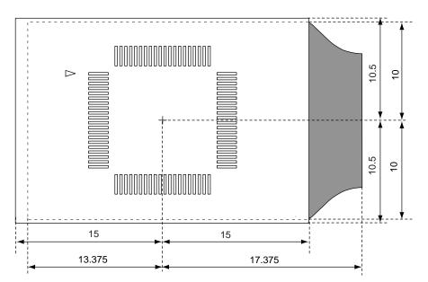
Figure B-6. The Restriction Domain on a Target System (Case of 80-pin GK Package)
