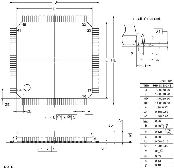
Each lead centerline is located within 0.13 mm of its true position at maximum material condition.
