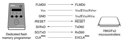
**Note** The above figure illustrates an example of wiring when using the clock output from the PG-FP5, FL-PR5, PG-FP4 or FL-PR4.
