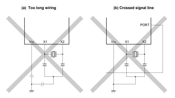
Figure 6-11. Examples of Incorrect Resonator Connection (1/2)
