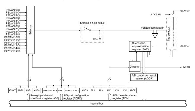
Figure 13-1. Block Diagram of A/D Converter
