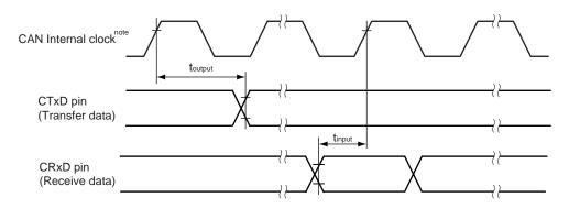
Internal delay time (tNODE) = Internal Transfer Delay (toutput) + Internal Receive Delay (tinput)
