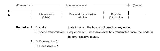
Usually, the intermission field is 3 bits. If the transmitting node detects a dominant level at the third bit of the intermission field, however, it executes transmission.
