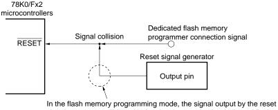
In the flash memory programming mode, the signal output by the reset signal generator collides with the signal output by the dedicated flash memory programmer. Therefore, isolate the signal of the reset signal generator.
