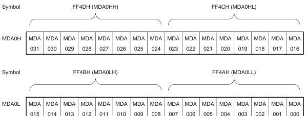
Cautions 1. MDA0H is cleared to 0 when an operation is started in the multiplication mode (when multiplier/divider control register 0 (DMUC0) is set to 81H).
