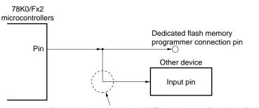
Figure 24-16. Malfunction of Other Device
