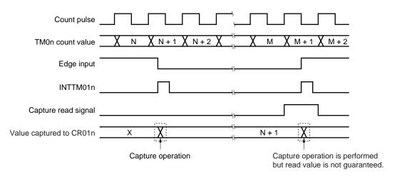
Figure 7-58. Timing of Holding Data by Capture Register
