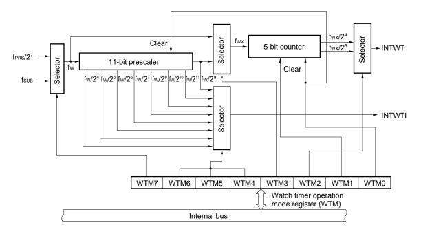
Figure 10-1. Block Diagram of Watch Timer
