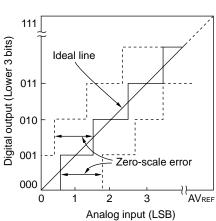
Figure 13-17. Zero-Scale Error
