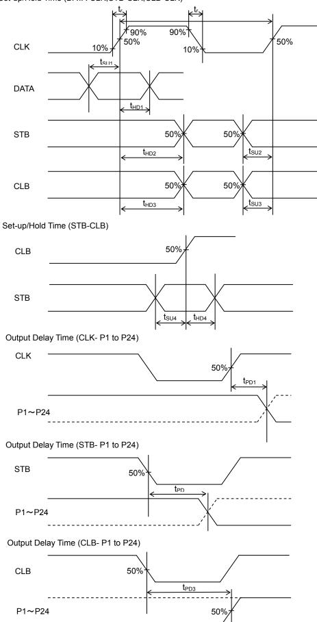
Figure 4. Switching Time Test Waveform
