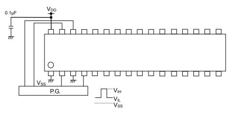
Figure 1. Input High/Low Voltage Measurement Circuit
