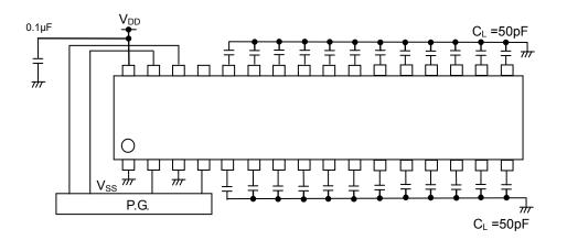
Figure 3. Switching Time Test Circuit
