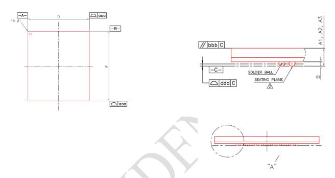
Figure 2- INAND Specification Top and Side View (Detail A)
