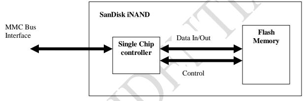
Figure 1 shows a block diagram of the SanDisk iNAND with MMC Interface.
