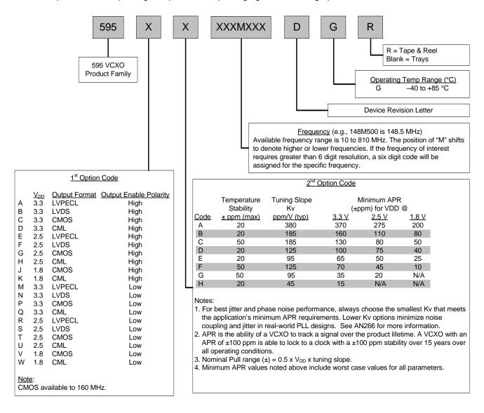
Example Part Number: 595AE148M500DGR is a 5 x 7 mm VCXO in a 6 pad package. The nominal frequency is 148.5 MHz, with a 3.3 V supply, LVPECL output, and Output Enable active high polarity. Temperature stability is specified as ±20 ppm and the tuning slope is 95 ppm/V. The part is specified for a –40 to +85 C° ambient temperature range operation and is shipped in tape and reel format.
