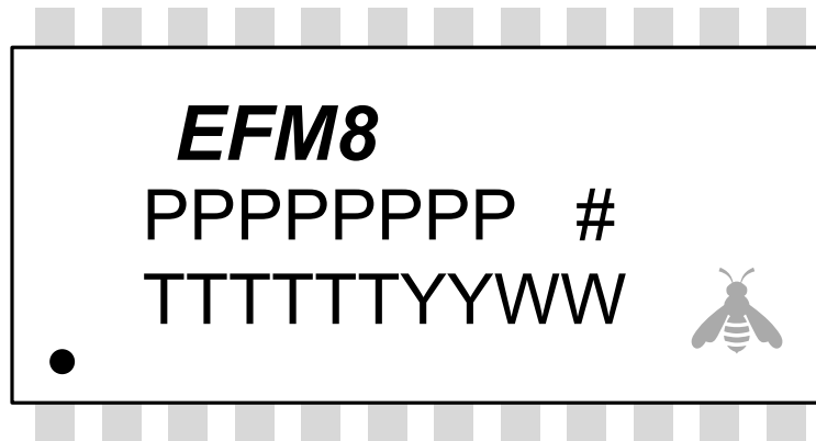
Figure 8.3. QSOP24 Package Marking
