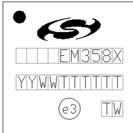
Figure 6.7. Part Marking for EM358x
