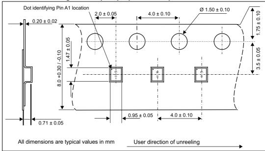
Figure 26. Flip Chip tape and reel specifications
