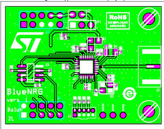
Figure 12. Application board EVB (2 layers)
