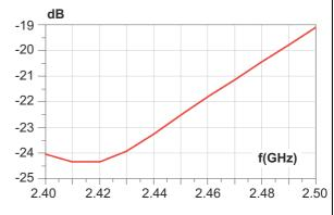
Figure 5. Insertion loss
