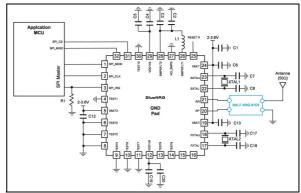
Figure 2. Application schematic with WLCSP type BlueNRG
