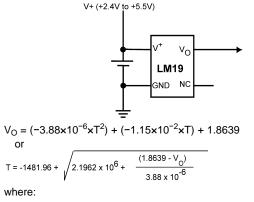
T is temperature, and  $V_{\rm O}$  is the measured output voltage of the LM19.
