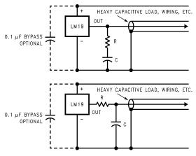
Either placement of resistor as shown above is just as effective.
