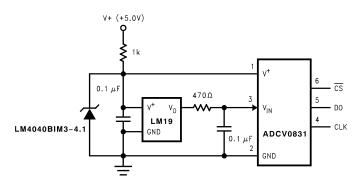
Figure 7. Suggested Connection to a Sampling Analog to Digital Converter Input Stage
