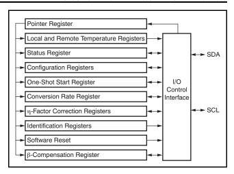
Figure 14. Internal Register Structure
