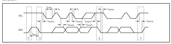
Figure 15. Two-Wire Timing Diagram
