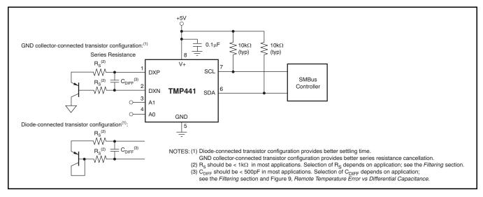
Figure 12. TMP441 Basic Connections
