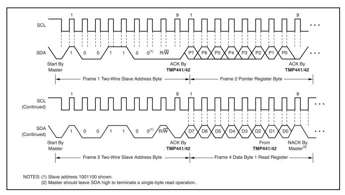
Figure 17. Two-Wire Timing Diagram for Single-Byte Read Format
