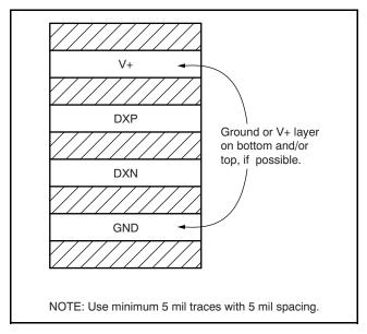
Figure 19. Suggested PCB Layer Cross-Section
