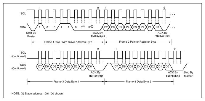
Figure 16. Two-Wire Timing Diagram for Write Word Format
