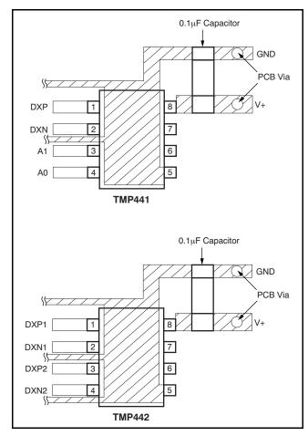
Figure 20. Suggested Bypass Capacitor Placement and Trace Shielding
