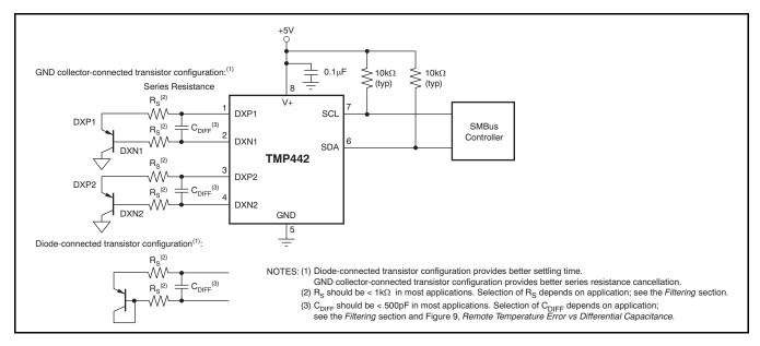
Figure 13. TMP442 Basic Connections
