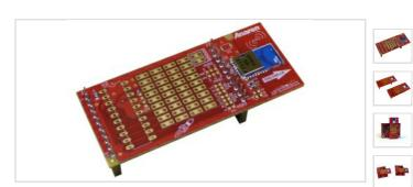
RF BoosterPack with the CC110L module from Anaren
