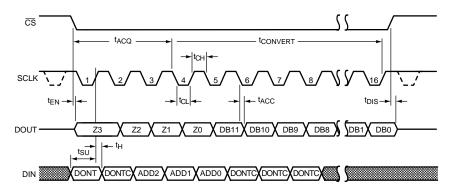
Figure 3. Serial Timing Diagram
