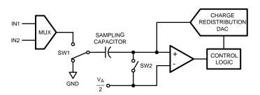
Figure 48. ADC122S051 in Hold Mode
