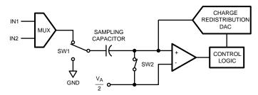
Figure 47. ADC122S051 in Track Mode
