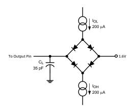
Figure 2. Timing Test Circuit
