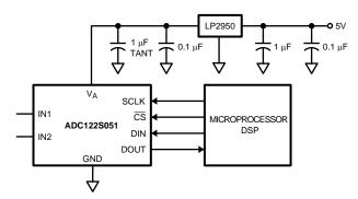
Figure 50. Typical Application Circuit
