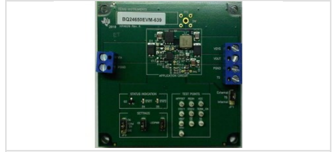
Evaluation Module Synchronous, Switch-Mode, Battery Charge Controller for Solar Power
