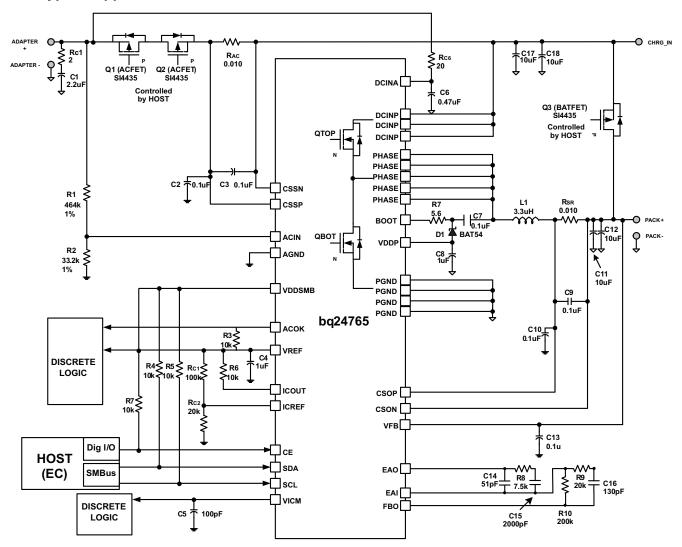
$V_{IN} = 20 \text{ V}, V_{BAT} = 4\text{-cell Li-Ion}, I_{CHARGE} = 4.5 \text{ A}, Idpm = 5 \text{ A}$
