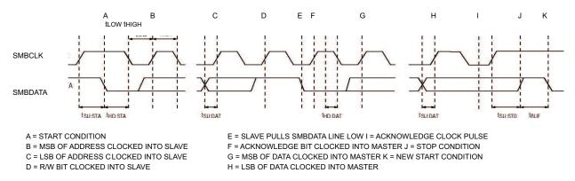
Figure 16. SMBus Read Timing
