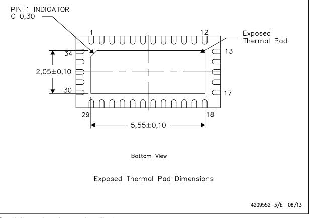
NOTE: All linear dimensions are in millimeters
