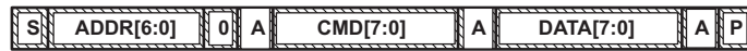
Figure 9. Attempt To Write a Read-Only Address (Nack After Data Sent By Master)
