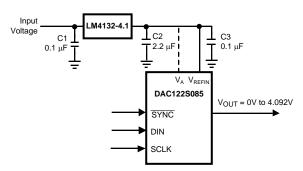
Figure 31. The LM4130 as a power supply
