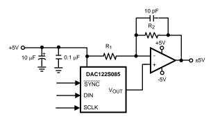
Figure 35. Bipolar Operation
