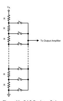
Figure 29. DAC Resistor String
