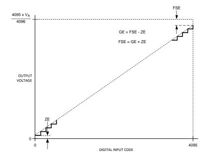
Figure 1. Input / Output Transfer Characteristic
