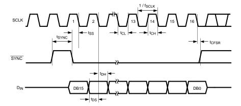
Figure 2. Serial Timing Diagram
