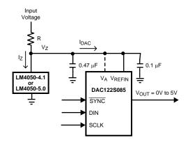
Figure 32. The LM4050 as a power supply
