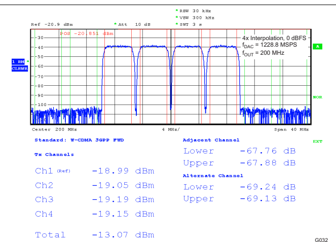
Figure 32. Four Carrier W-CDMA Test Model 1
