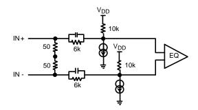
Figure 6. Simplified Receiver Input Termination Circuit
