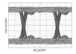
Figure 14. Equalized Signal (32 In Tyco XAUI Backplane, 3.125 Gbps, PRBS7, 0x07 Setting)
