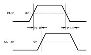
Figure 3. Propagation Delay Timing Diagram
