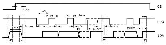
Figure 7. SMBus Timing Parameters
