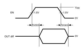
Figure 5. Enable (EN) Delay Timing Diagram
