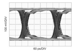
Figure 12. Equalized Signal (40 In FR4, 3.2Gbps, PRBS7, 0x07 Setting)
