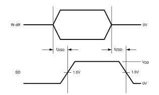
Figure 4. Signal Detect (SD) Delay Timing Diagram
