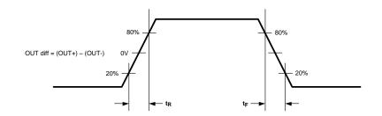
Figure 2. CML Output Transition Times
