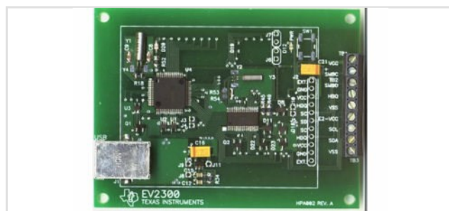
USB-Based PC Interface Board for Battery Fuel Gauge Evaluation, Gas Gauge SMBus or HDQ
