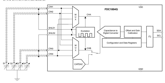
Figure 12. Differential Configuration
