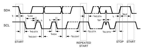
Figure 1. I<sup>2</sup>C Timing
