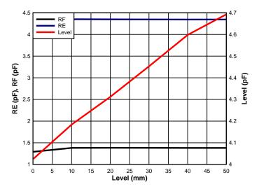
Figure 16. Electrodes' Capacitance vs. Liquid Level
