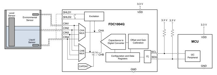
Figure 15. FDC1004Q (Liquid Level Measurement)
