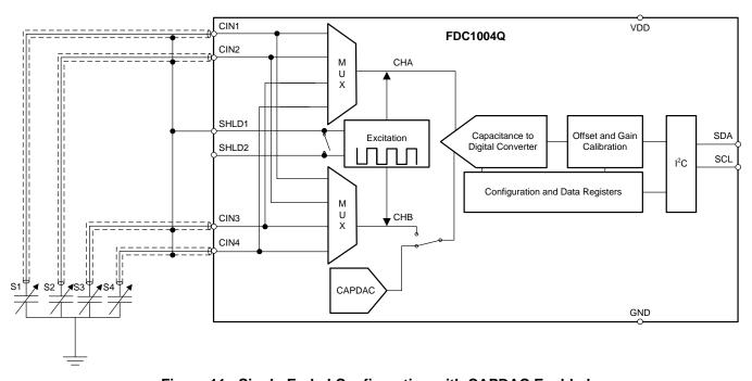
Figure 11. Single-Ended Configuration with CAPDAC Enabled
