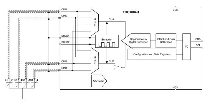
Figure 10. Single-Ended Configuration with CAPDAC Disabled
