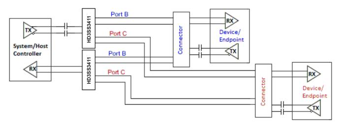
Figure 5. AC Coupling Capacitors on Host TX and Endpoint TX
