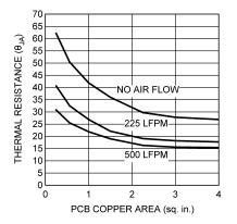
Figure 32. Thermal Resistance vs PCB Area (4 Layer Board)
