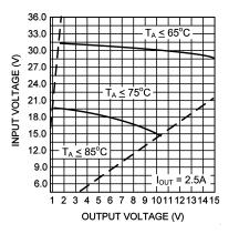
Figure 31. Safe Thermal Operating Areas ( $I_{OUT} = 2.5A$ )
