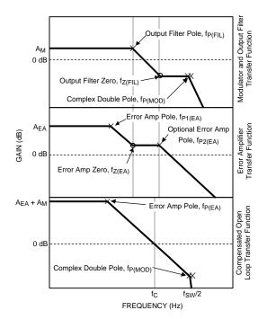
Figure 25. LM20323 Loop Compensation
