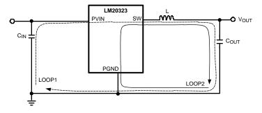
Figure 33. Schematic of LM20323 Highlighting Layout Sensitive Nodes
