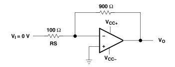
Figure 2. Noise-Test Circuit
