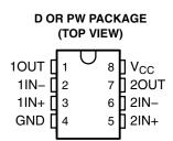
This device consists of two independent, high-gain, frequency-compensated operational amplifiers designed to operate from a single supply over a wide range of voltages. Operation from split supplies is possible as long as the difference between the two supplies is 3 V to 26 V (3 V to 32 V for V-suffix devices), and  $V_{CC}$  is at least 1.5 V more positive than the input common-mode voltage. The low supply-current drain is independent of the magnitude of the supply voltage.
