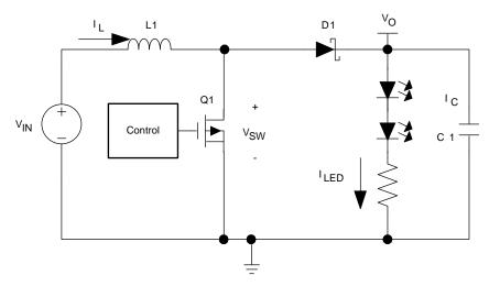
Figure 10. Simplified Boost Topology Schematic
