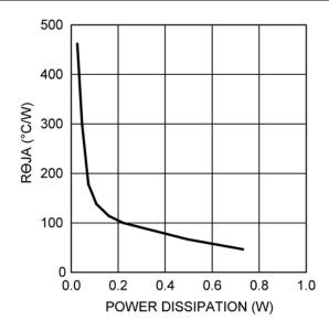
Figure 38. R<sub>0JA</sub> vs Internal Dissipation
