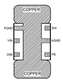
Figure 32. Boost PCB Layout Guidelines
