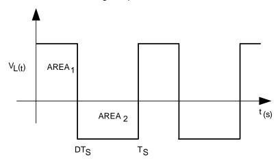
Figure 16. Inductor Volt-Second Balance Waveform
