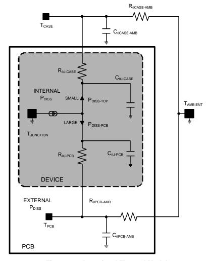
Figure 36. Associated Thermal Model
