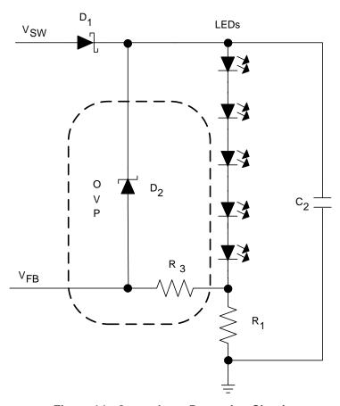
Figure 14. Overvoltage Protection Circuit
