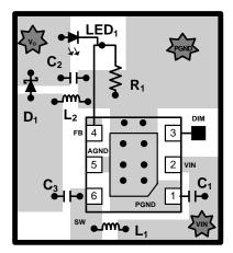
The layout guidelines described for the LM3410 boost-converter are applicable to the SEPIC OLED Converter. This is a proper PCB layout for a SEPIC Converter.
