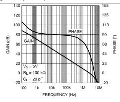
Figure 3. Open-Loop Gain and Phase With Resistive Load
