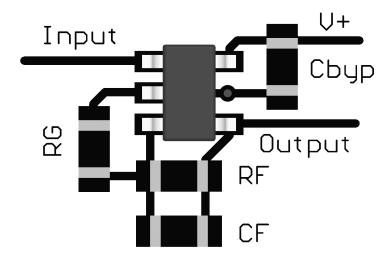
Figure 32. SOT-23 Layout Example
