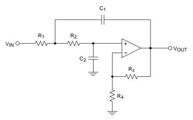
Figure 29. Two Pole Sallen-Key Low Pass Filter
