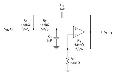
Figure 30. 1kHz Sallen-Key Low Pass Filter with Values
