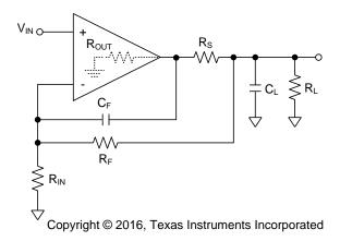
Figure 27. In the Loop Compensation
