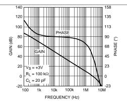
Figure 1. Open-Loop Gain and Phase With Capacitive Load
