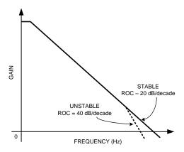
Figure 26. Gain vs Frequency for an Op Amp
