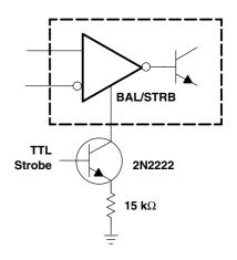
NOTE: Do not connect strobe pin directly to ground, because the output is turned off whenever current is pulled from the strobe pin.
