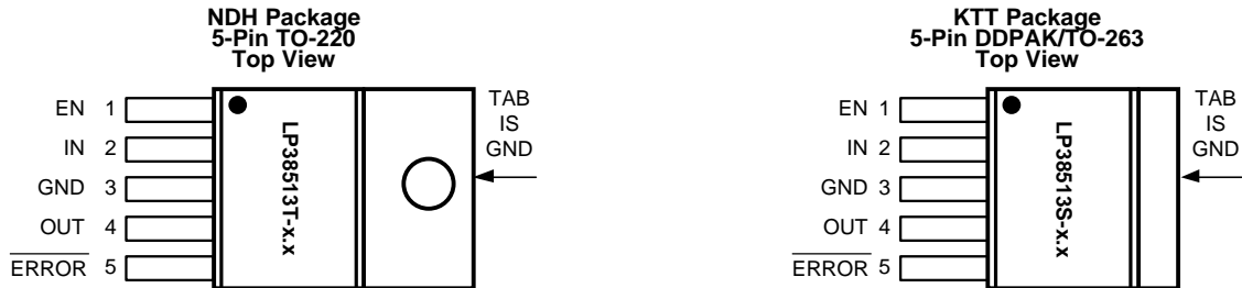
Pin Functions for TO-220 and DDPAK/TO-263 Packages
