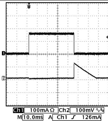
V<sub>IN</sub> = 3.6 V      V<sub>OUT</sub> = 2.6 V      0 to 150-mA Load
