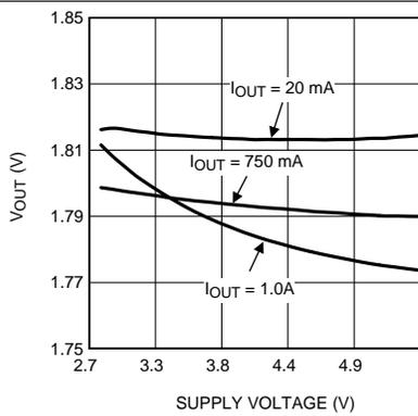
$V_{OUT} = 1.8\text{ V}$
