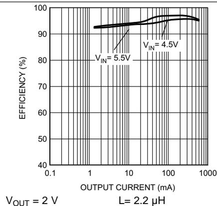
**Figure 48. Efficiency vs Output Current (PWM-to-PFM Mode)**
