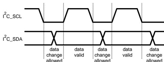
Figure 39. I<sup>2</sup>C Signals: Data Validity
