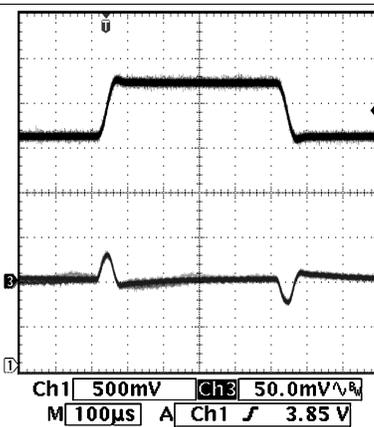
V<sub>IN</sub> = 3.6 to 4.2 V      V<sub>OUT</sub> = 2.6 V      300-mA Load
