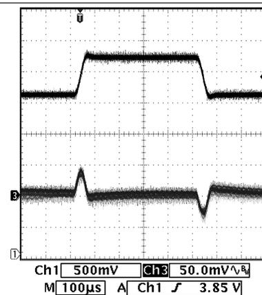
V<sub>IN</sub> = 3.6 to 4.2 V      V<sub>OUT</sub> = 3.3 V      300-mA Load
