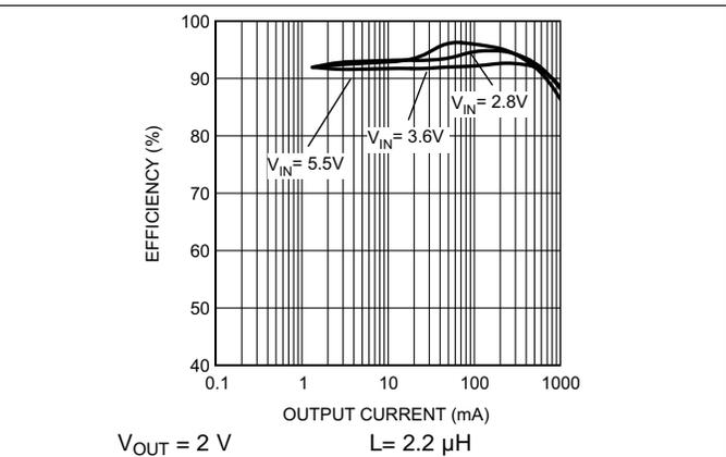
Figure 17. Efficiency vs Output Current (PWM-to-PFM Mode)
