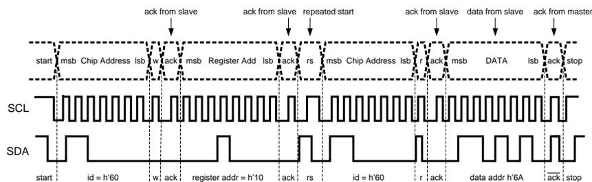
**Figure 43. I<sup>2</sup>C Read Cycle**
