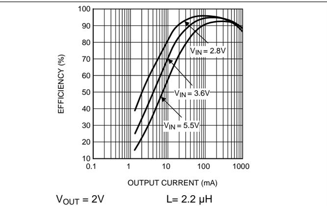
Figure 15. Efficiency vs Output Current (Forced PWM Mode)
