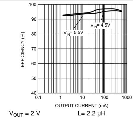
Figure 21. Efficiency vs Output Current (PWM-to-PFM Mode)
