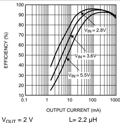
**Figure 47. Efficiency vs Output Current (Forced PWM Mode)**
