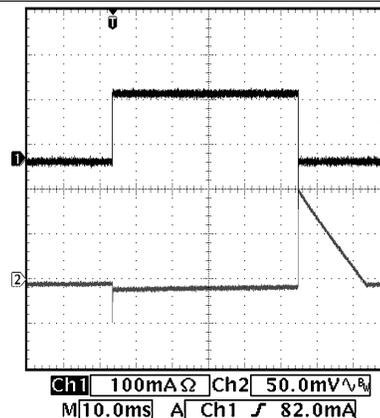
V<sub>IN</sub> = 3.6 V      V<sub>OUT</sub> = 3.3 V      0 to 150-mA Load
