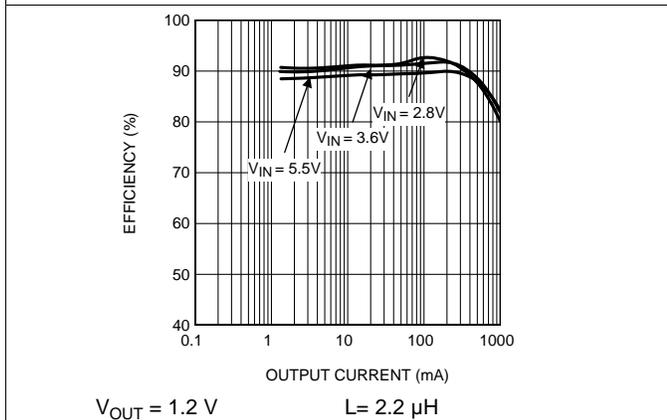
Figure 16. Efficiency vs Output Current (PWM-to-PFM Mode)
