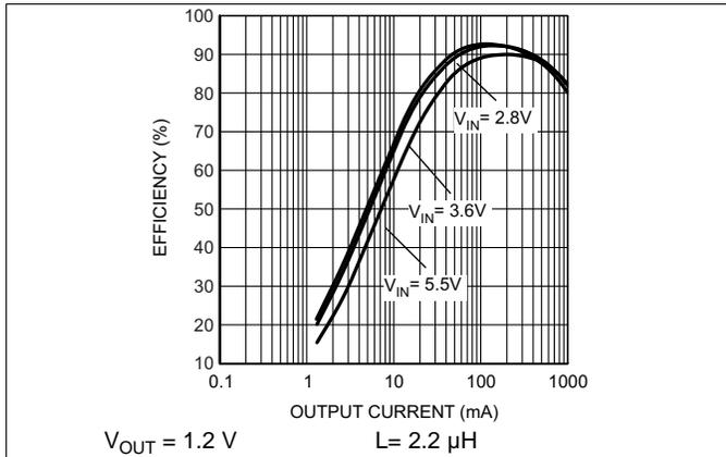
Figure 14. Efficiency vs Output Current (Forced PWM Mode)
