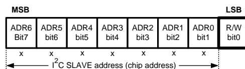
Figure 18. I 2 C Chip Address
