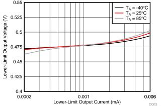
Figure 2. Output Low Voltage ( $V_{OL}$ ) vs. Output Low Current ( $I_{OL}$ ) for SCL0 at Different Temperatures for  $V_{CC}$ = 5 V
