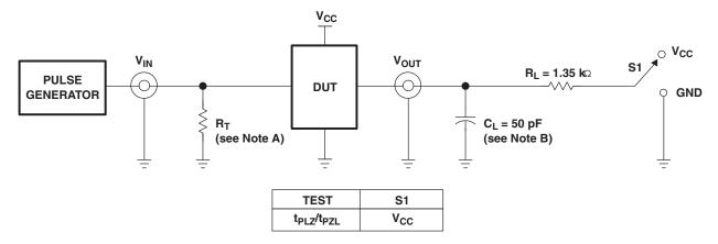
**TEST CIRCUIT FOR OPEN-DRAIN OUTPUT**
