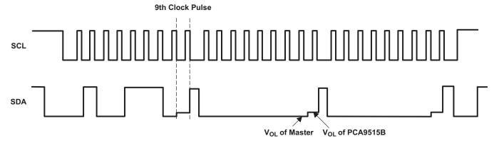
Figure 6. Bus 0 Waveforms
