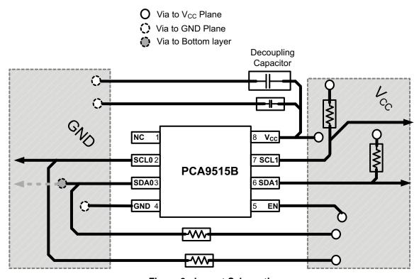
Figure 8. Layout Schematic
