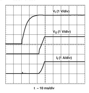
Figure 10. Power-Up Waveforms
