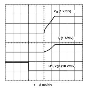
Figure 12. Power Up Response From Inhibit Control
