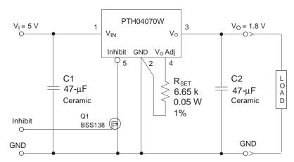
Figure 11. On/Off Inhibit Control Circuit
