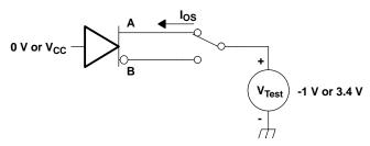
Figure 4. Driver Short-Circuit Test Circuit
