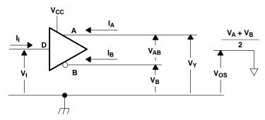
Figure 1. Driver Voltage and Current Definitions
