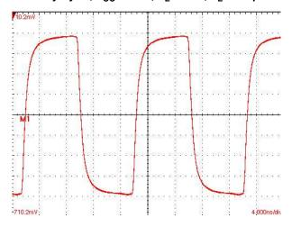
Output duty cycle = 50.01%. Vertical scale = 142 mV/div Horizontal scale = 4 ns/div
