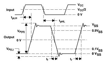
NOTE: All input pulses are supplied by a generator having the following characteristics:  $t_r$  or  $t_f \le 1$  ns, frequency = 1 MHz, duty cycle =  $50 \pm 5\%$ .
