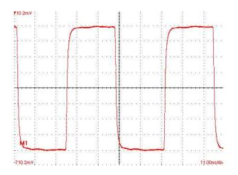
Output Duty cycle = 49.97%. Vertical scale = 142 mV/div Horizontal scale = 11 ns/div
