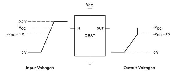
NOTE A: If the input high voltage ( $V_{IH}$ ) level is greater than or equal to  $V_{CC} - 1$  V, and less than or equal to 5.5 V, the output high voltage ( $V_{OH}$ ) level will be equal to approximately the  $V_{CC}$  voltage level.
